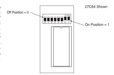
Figure 3.1 Channel DIP Switch Setting
