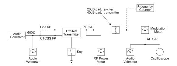
Figure 3.2 T836/837 Test Equipment Set-up
